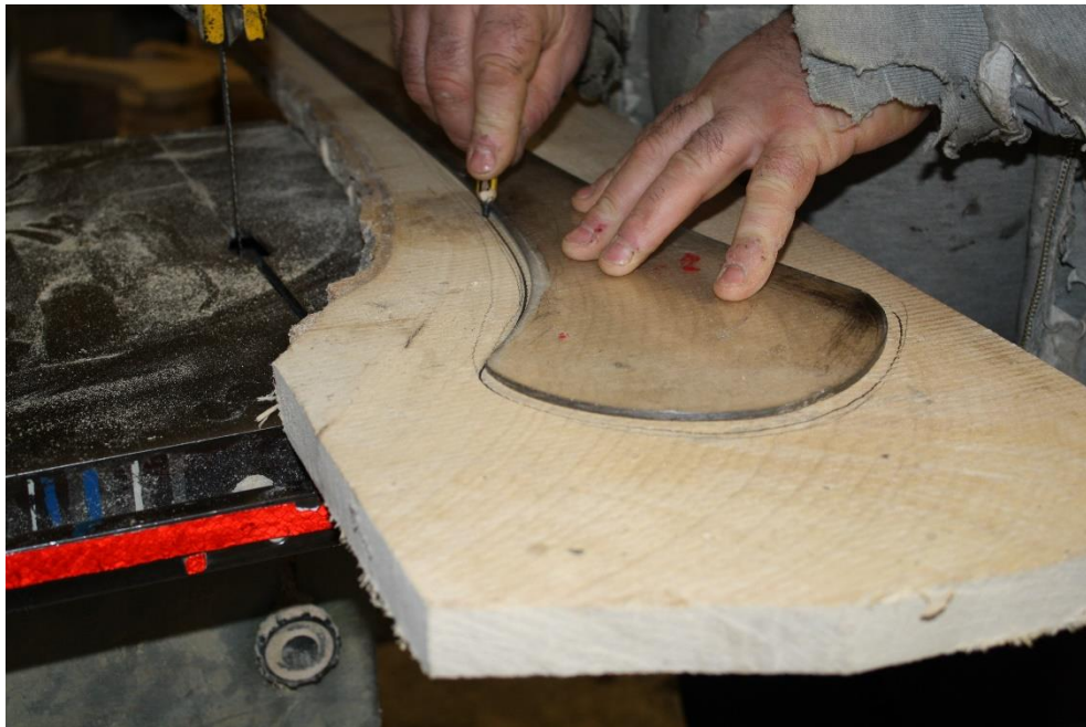
Figure 4: The outline of the hurl is marked on the plank (Photograph by the author, 2019).
