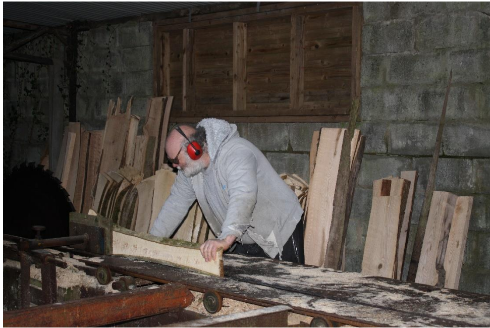
Figure 3: Cutting the timber into planks at the circular saw (Photograph by the author, 2019).
