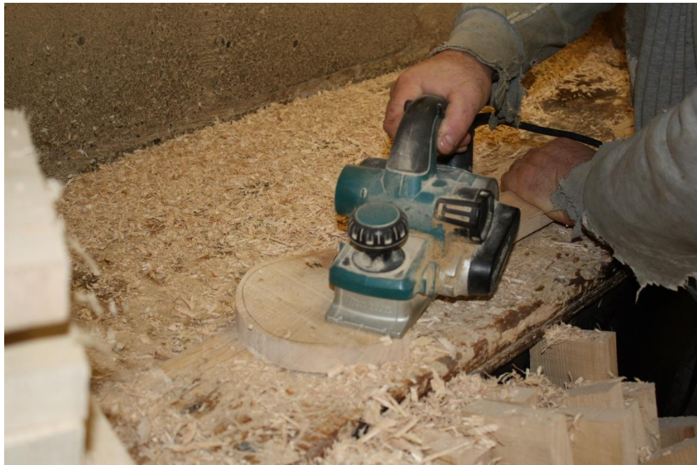
Figure 5: Planing the hurl at the workbench (Photograph by the author, 2019).
